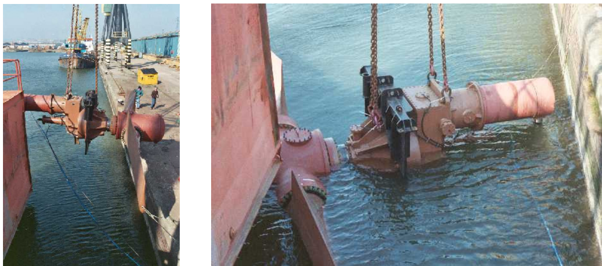
Figure 9: Submergence test for the power train on the quayside at Swansea.
