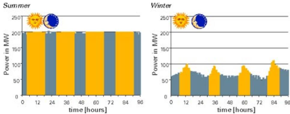
**Fig. 10 Results of simulation runs (electric power output versus time of day) of a 200 MW solar tower with 25 percent of collector area covered by water-filled bags as additional thermal storage (weather data from [17])**
