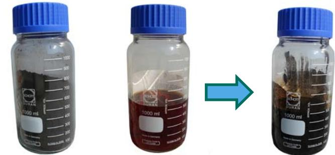
Koks + Pyrolyseöl ⇨ BioSyncrude
