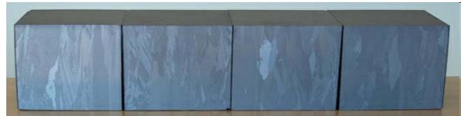
Bricks of multicrystalline silicon produced via the Vertical Gradient Freeze method at SIMTEC.
