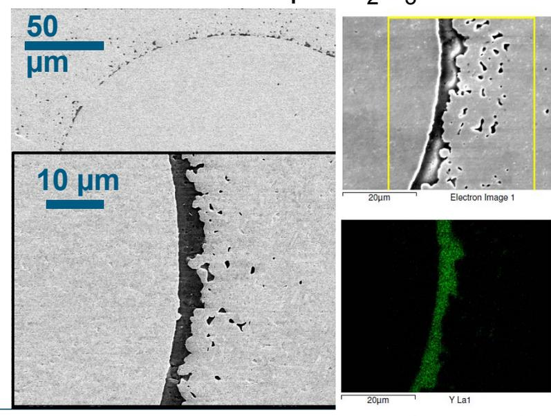
2.5  $\mu\text{m}$   $\text{Y}_2\text{O}_3$  interface
