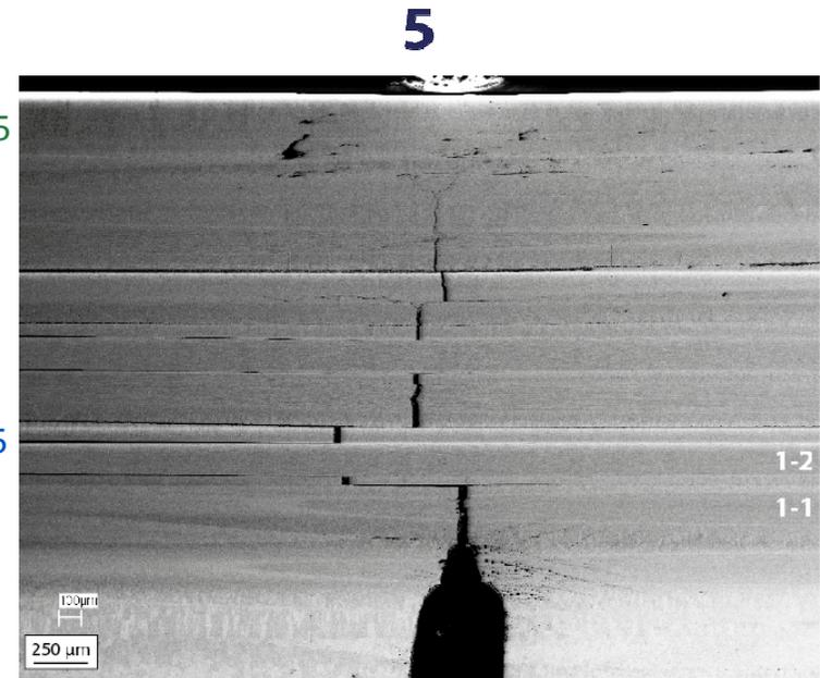
**Controlled** crack propagation + **rising load bearing capacity**
