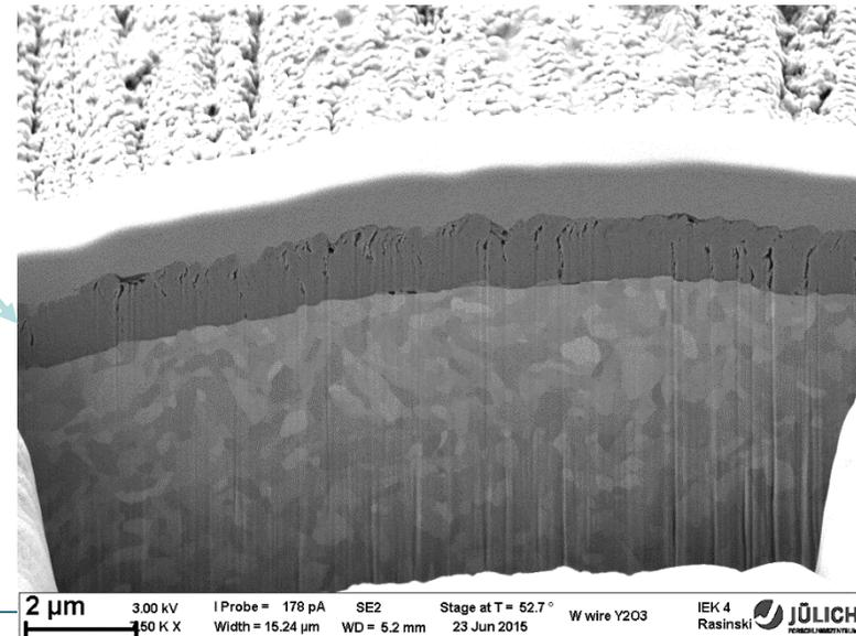
**High quality, homogeneous distributed  $Y_2O_3$  coating for the short fibers can be prepared by magnetron sputtering**
