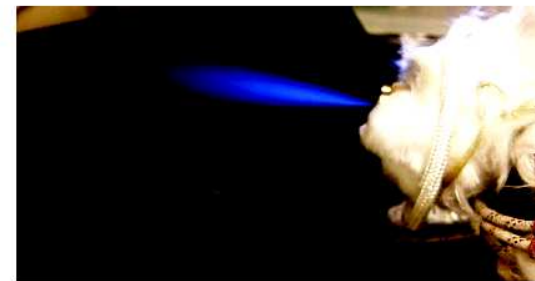
Fig. 4 Supercritical saltwater spray plumes illuminated with white light. A: micron-sized droplets; B, C: submicron-sized salt crystals. Blue color due to Rayleigh scattering of blue light by nanometer-sized salt particles.
