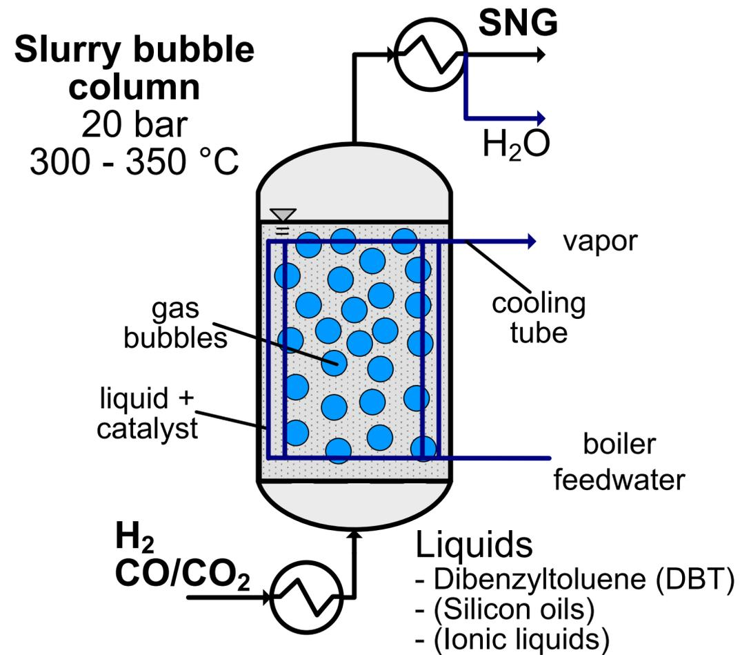
Figure 1: Schematic of a three-phase methanation reactor.
