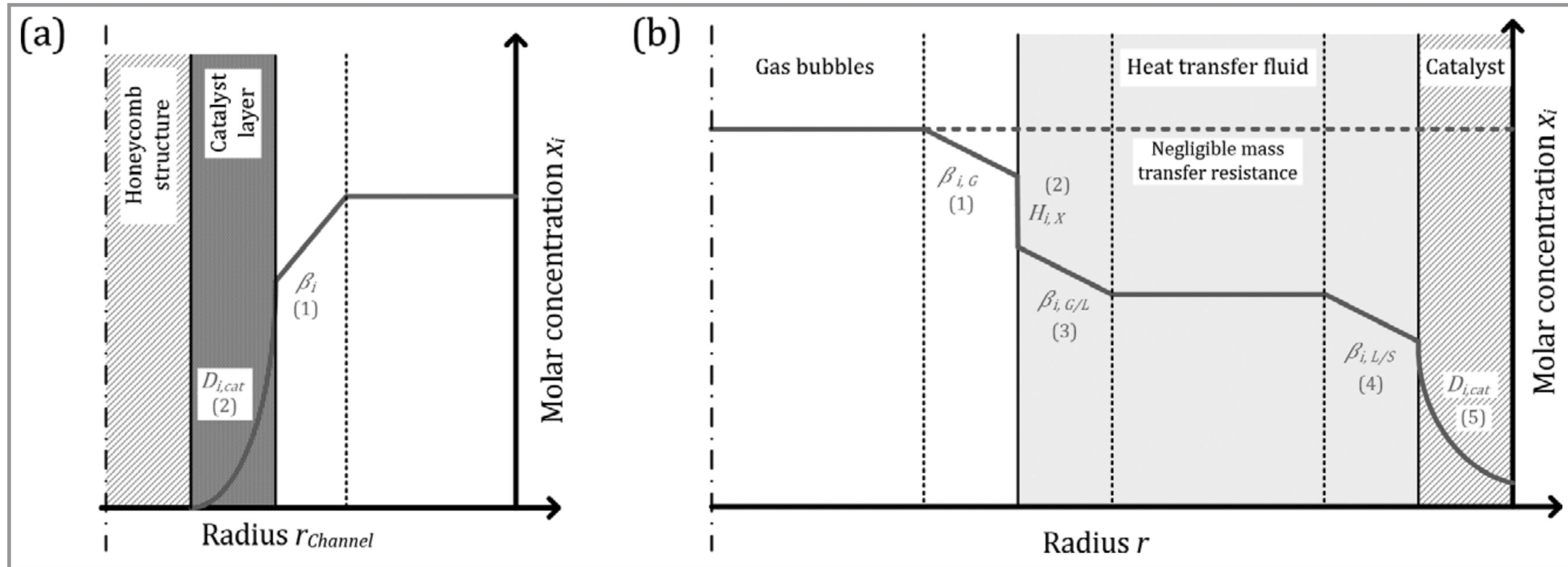
**Figure 3.** Mass transfer phenomena in the honeycomb reactor (a) and the three-phase reaction system (b) based on theoretical considerations.
