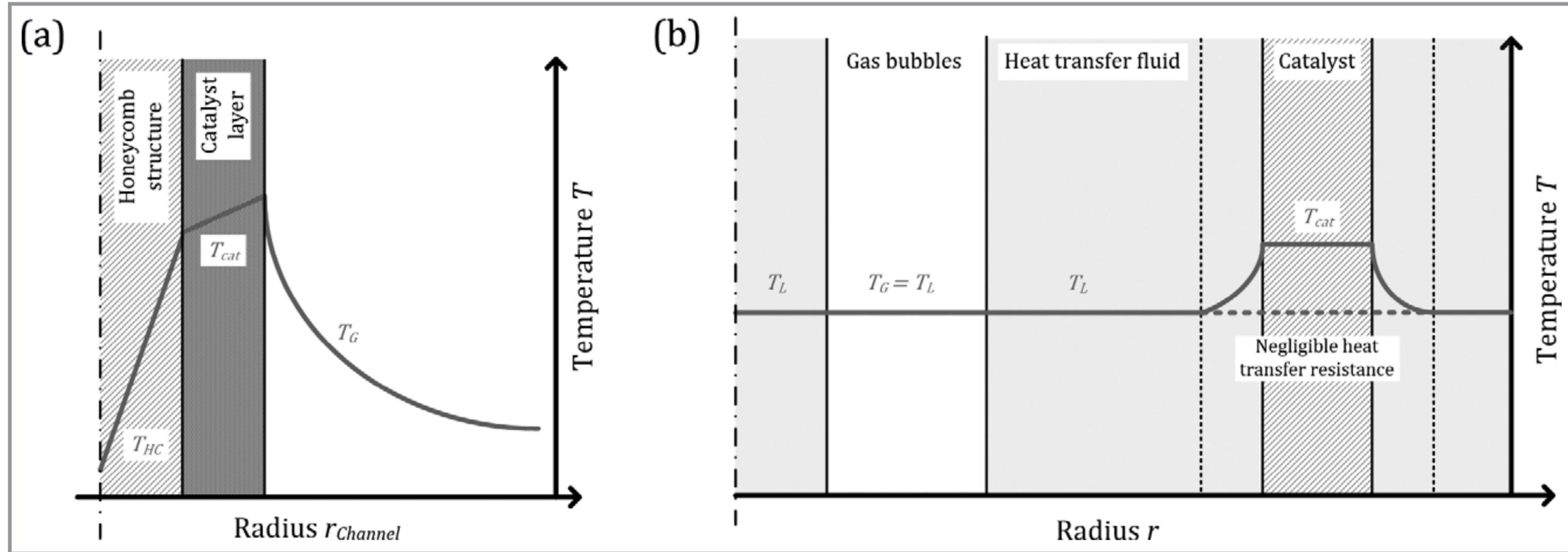
**Figure 4.** Heat transfer phenomena in the honeycomb reactor (a) and the three-phase reaction system (b) based on theoretical considerations.
