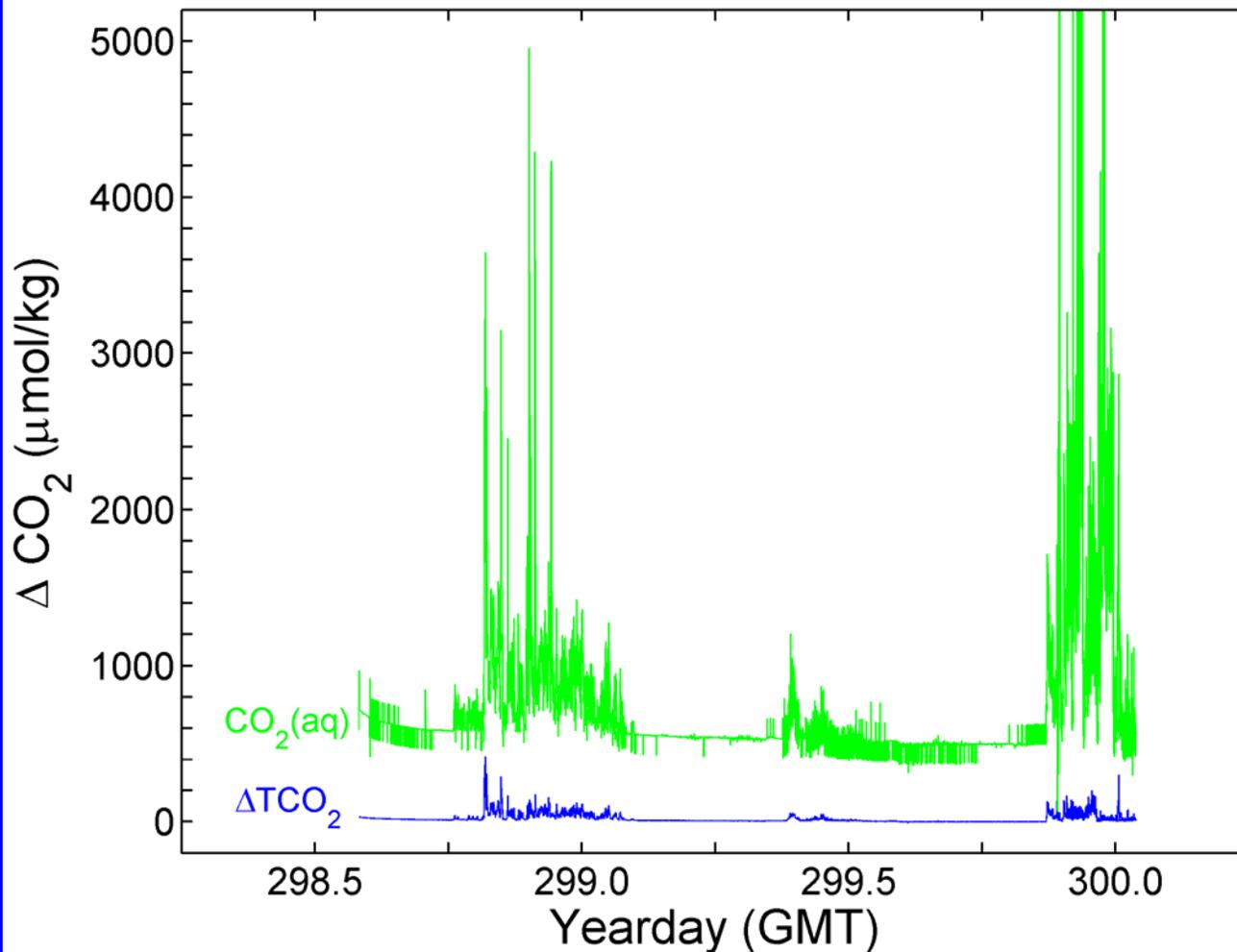
*The record of  $\text{CO}_2\text{aq}$  deduced from the conductivity record, and the change in  $\text{TCO}_2$  as  $\text{HCO}_3^-$ . Both sensors are about 30cm distant from the  $\text{CO}_2$  source. The  $\text{CO}_2\text{aq}$  signal clearly dominates, and the ratio will shift downstream as the hydration-ionization process occurs. From Brewer et al. 2004.*
