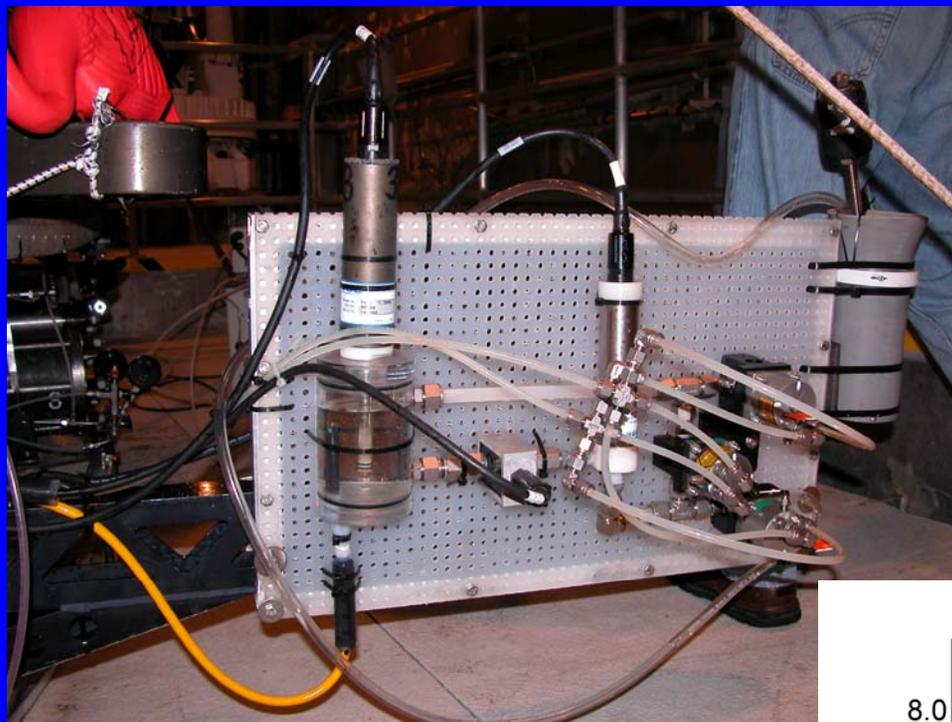
*A simple kinetic test. Sea water is drawn into the pH cell, the valves are closed and the time to reach pH equilibrium in the flow loop is observed.*
