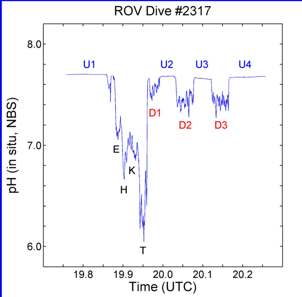
*pH values were calibrated and reported on the NBS scale. The probe was placed upstream, inside the box, and downstream.*
