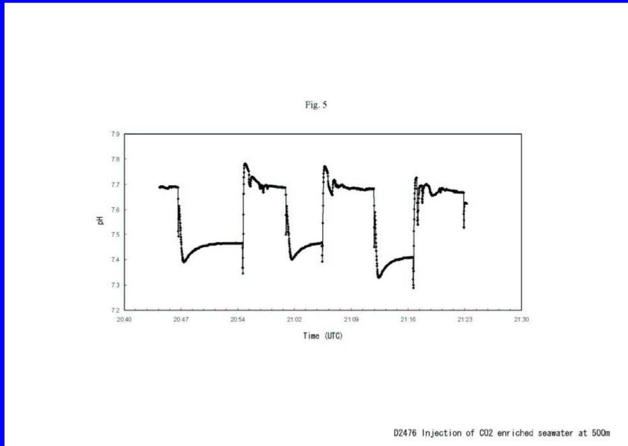
*The shape of the curve differs from acid injection and is consistent with removal of excess  $\text{HCO}_3^-$ . This requires a volume increase, and the reaction at depth is slower than for acid addition – but still far faster than at 1 atm.*
