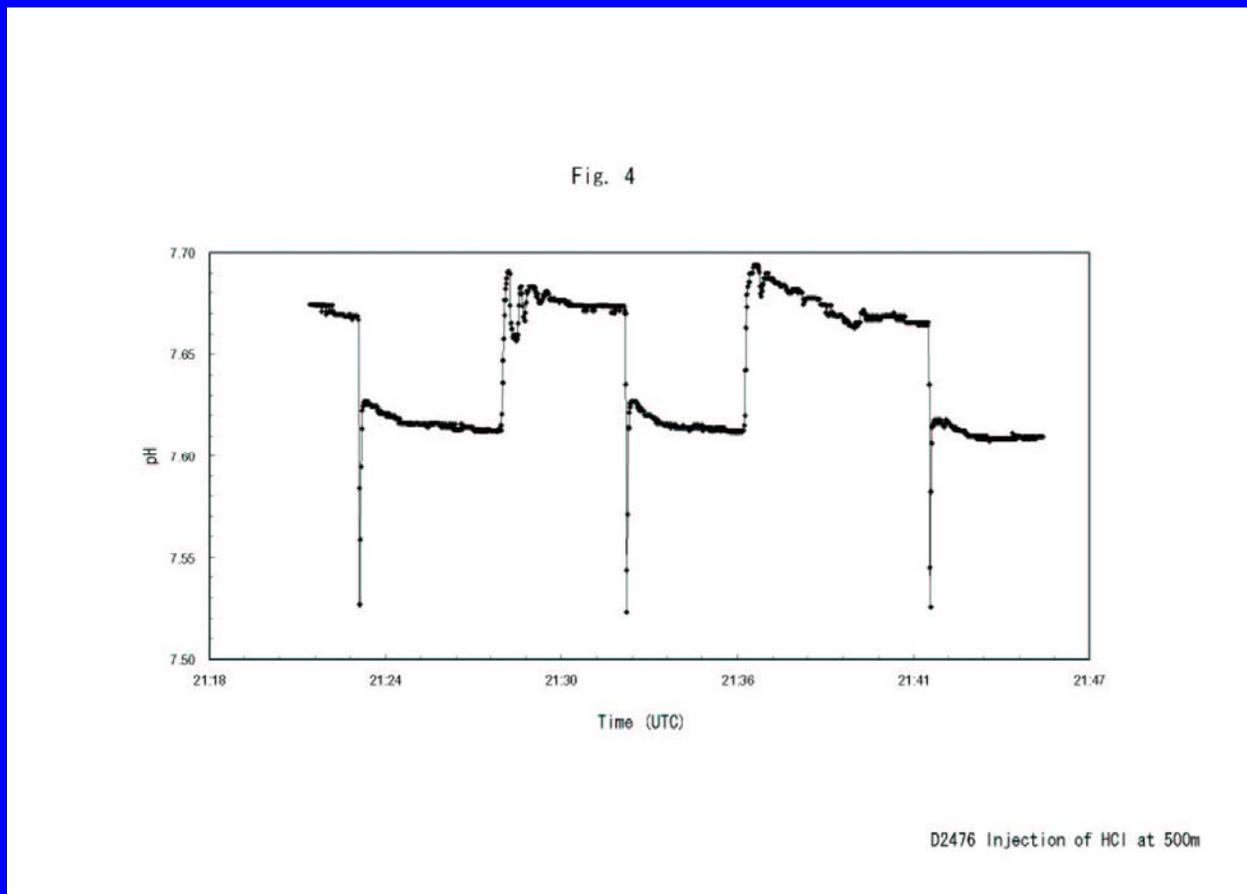
***The data are consistent with formation of an intense cloud of  $\text{CO}_2$  at the injection tip, followed by rapid mixing and hydration of the excess  $\text{CO}_2$  to form  $\text{HCO}_3^-$ . This reaction has a volume decrease, and is accelerated by pressure.***
