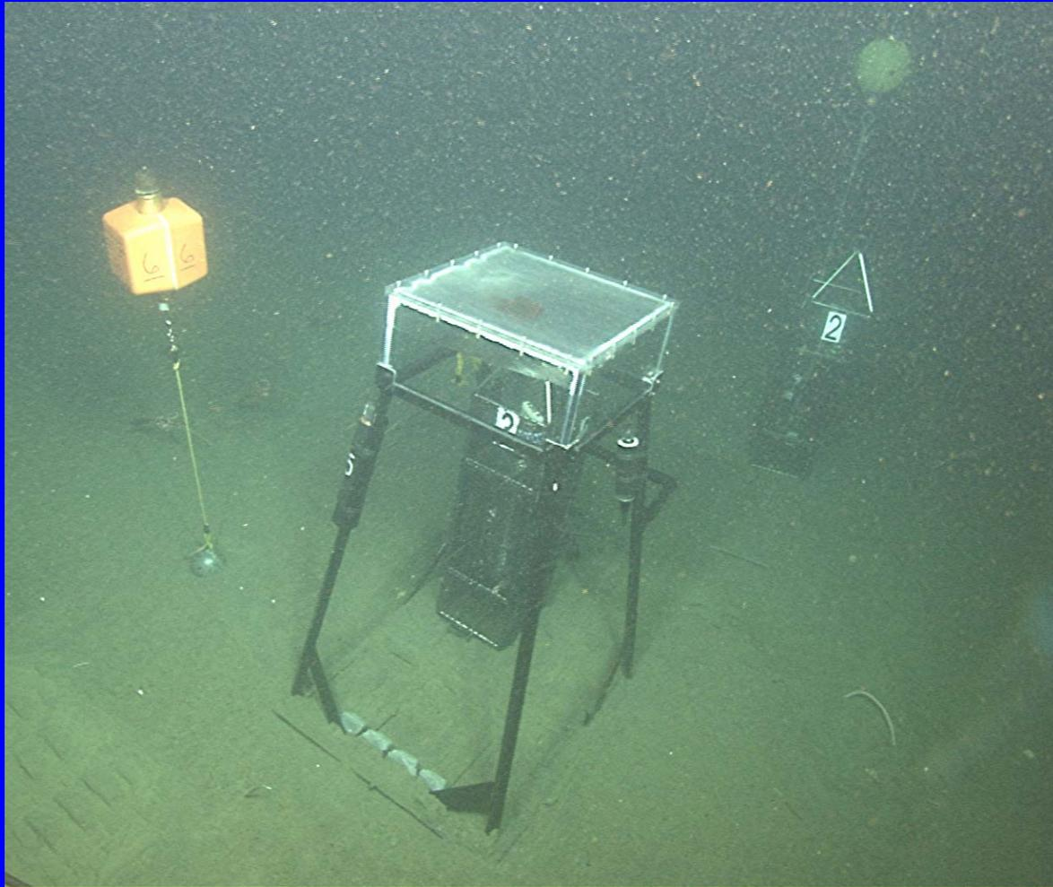
***The experiment was designed to test the signature of the dense low pH plume from the CO<sub>2</sub> pool.***
