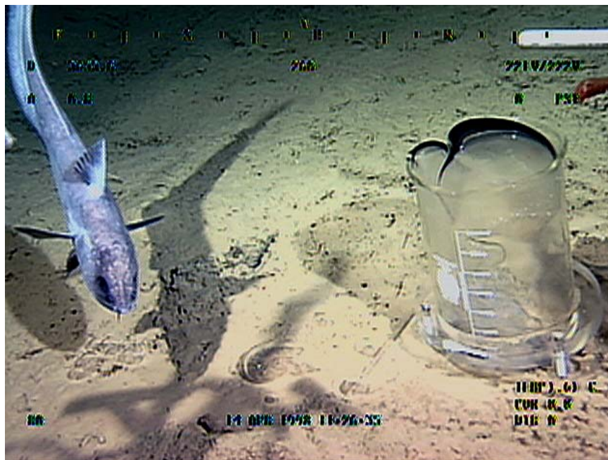
Figure 4. A 4L beaker filled with liquid CO 2 at a depth of 3,600m is inspected by a Pacific Grenadier fish. The CO 2 has reacted with sea water to form a hydrate, and the volume expansion has caused spill over of the liquid. From Brewer et al. (1999).
