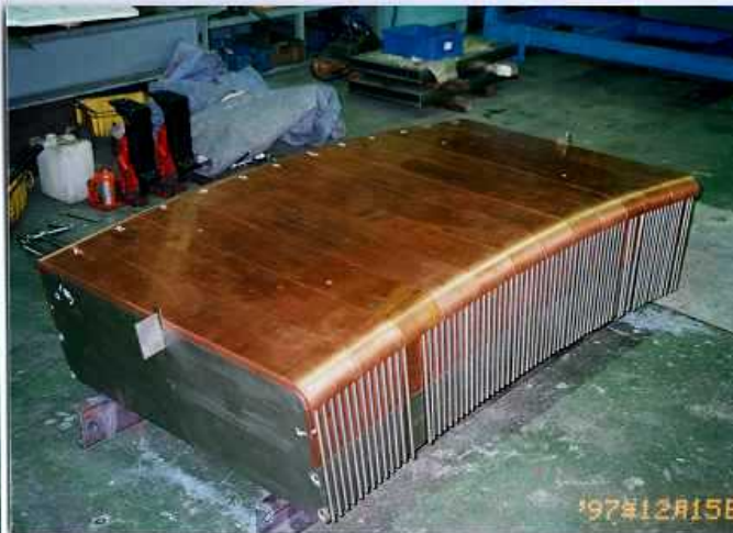
Final assembly of FW and shield block
