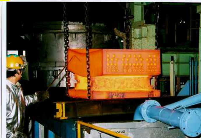
Steel block after solution heat treatment (1010-1054 °C)
