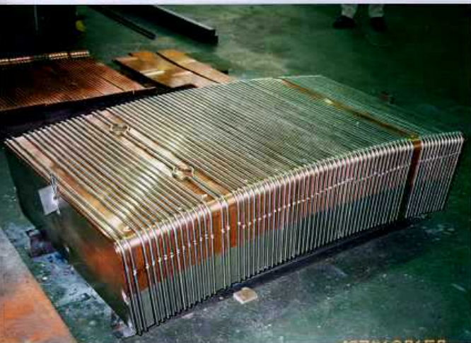
Assembly of steel tubes and DS Cu plates
