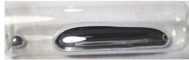
Liquid mercury in glass capsule
