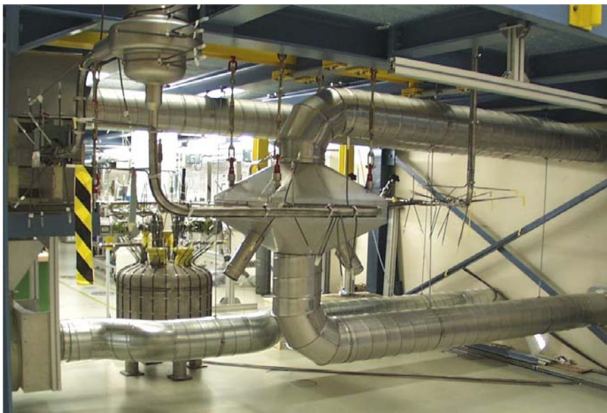
MHD Pump and Recuperator
