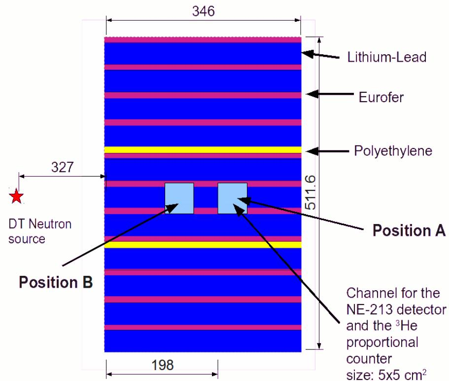
Two measurement position have been used. Only one channel was present at a time.
