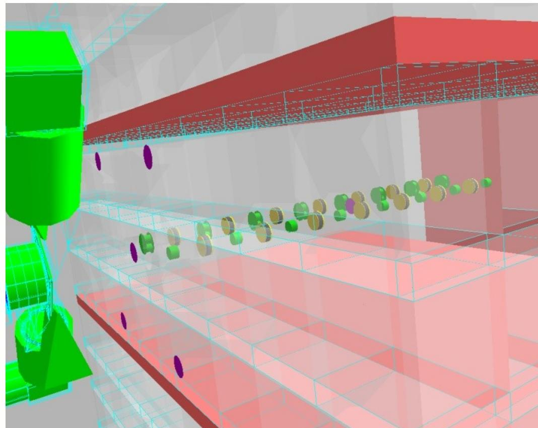
Mock-up consists of layers of LiPb, Eurofer and polyethylene
