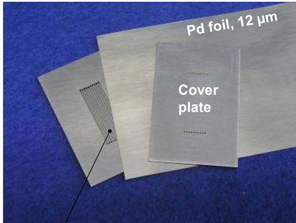
Laser welded unit (Pd foil size: 40 x 27 mm 2 )
