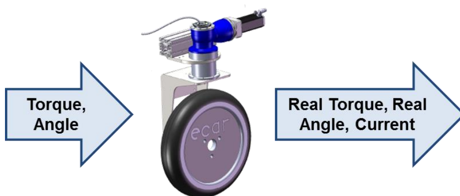
Fig.7. eCorner as highly integrated smart component.
