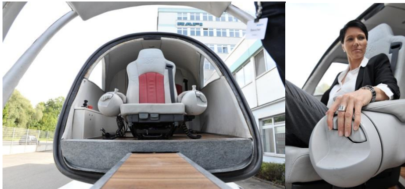
Fig. 11. Sphere sidesticks integrated in the driver's seat
