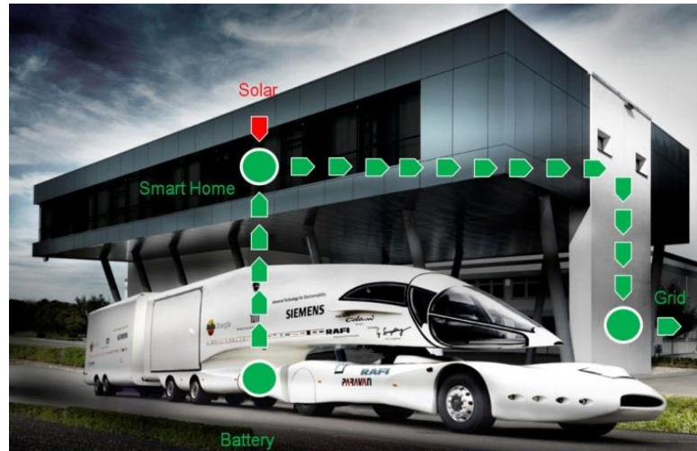
Fig. 1. Electric vehicles can be utilized in a form of a large virtual battery to stabilize the grid.
