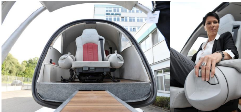
Fig. 11. Sphere sidesticks integrated in the driver's seat
