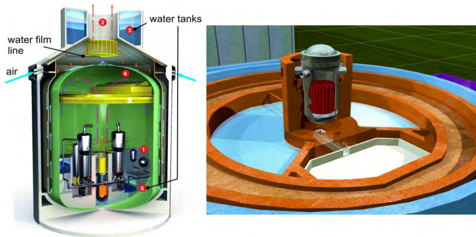
Fig. 10: Different design based safety provisions to control core meltdown situations: in-vessel retention strategy [17, left] and core-catcher of the EPR [18, right].
