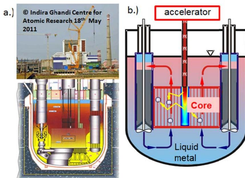
**Figure 18:** (a) Sodium cooled fast reactor currently erected in India and core cross-section. (b) Schematical cross-sectional cut of an eutectic PbBi cooled sub-critical ADS reactor developed at SCK-CEN, Belgium.
