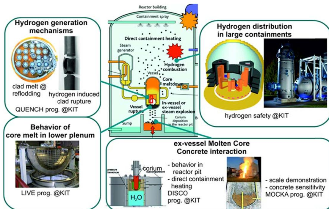
**Figure 12:** Potential containment phenomena occurring in a case of a severe accident [19] and associated R&D experimental programs at KIT.
