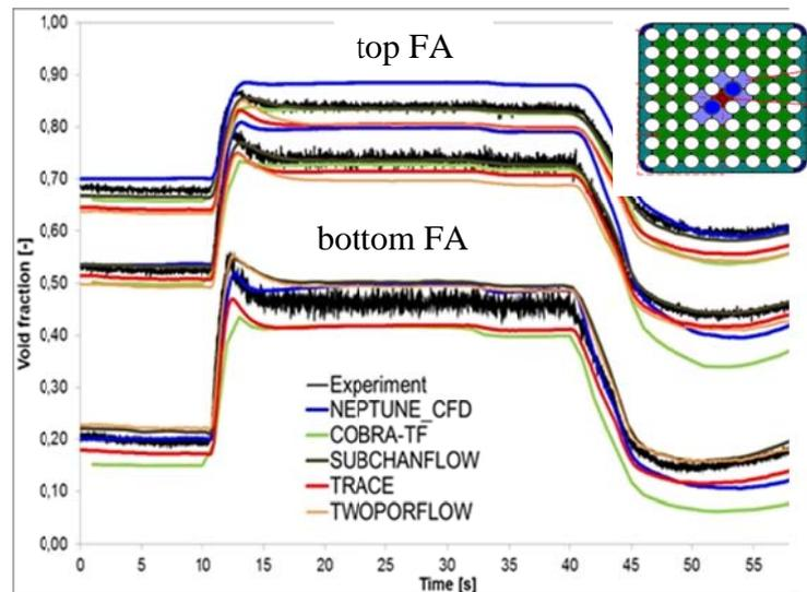
**Figure 4:** Computed void fraction distributions at three different axial heights by different codes during a pump trip in comparison with the experiment [12].
