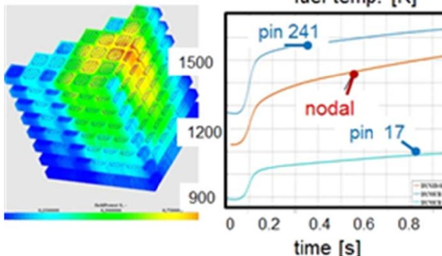
**Figure 8:** Pin based solution of the power distribution (left) during a rod ejection accident (REA). Comparison of the temporal evolution of fuel pin temperatures for a pin-based solution compared to a nodal solution [14].
