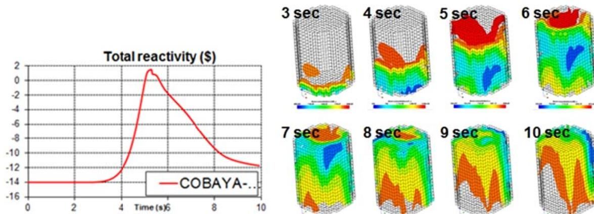
**Figure 5:** Thermal-hydraulics – neutronic coupling for a boron dilution transient in which deborated water (blue) enters the core leading to first to reactivity increase and by feedbacks afterwards to a reduction [13] and corresponding reactivity change (left).
