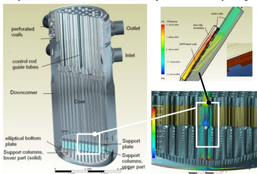
**Figure 3:** Transfer from micro-scale CFD (top right) to meso scale (bottom right) and then to reactor scale (left.).
