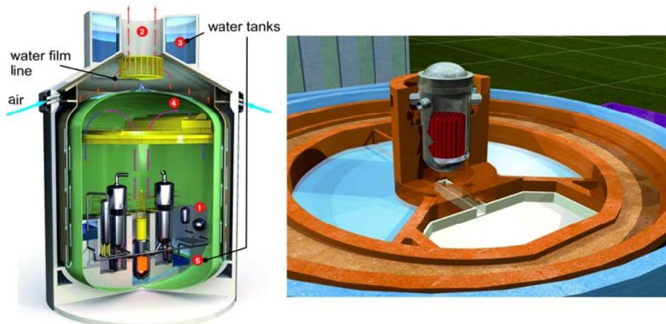
**Figure 11:** Different design based safety provisions to control core melt-down situations: in-vessel retention strategy [17, left] and core-catcher of the EPR [18, right].
