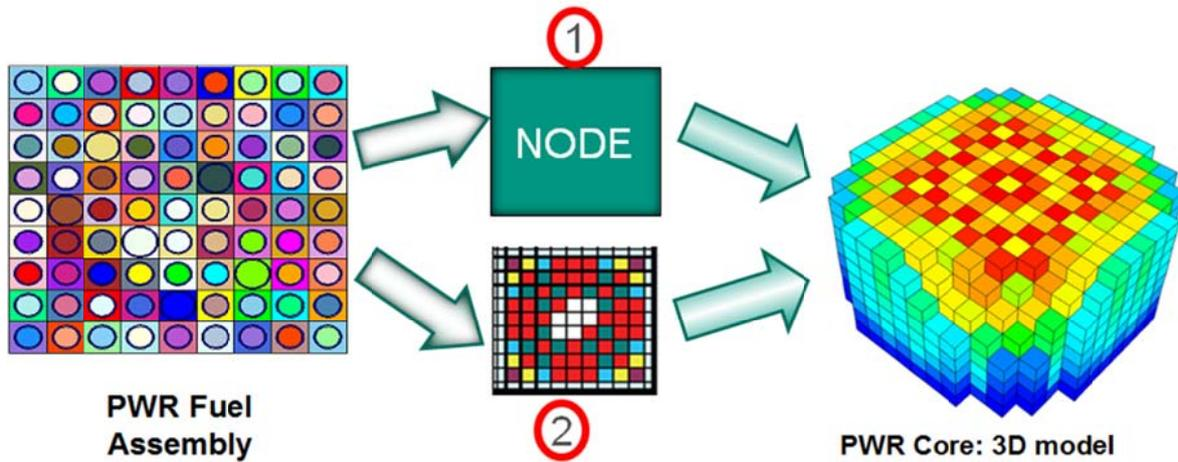
**Figure 7:** Different options for high fidelity coupled N-TH computations. Path (1) via homogenization and subsequent PPR methods. Route (2) full pin-based solutions.
