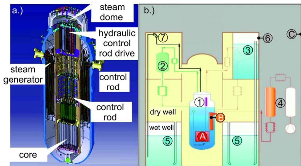
**Figure 14:** (a) integral core design of the CAREM 25 reactor. CAREM 25 safety systems: 1=first shutdown system, 2=second shutdown system, 3=residual heat removal system primary system, 4=emergency injection system, 5=pressure suppression pool, 6=containment, 7=safety valves, A=core, B=steam generators, C=reactor building.
