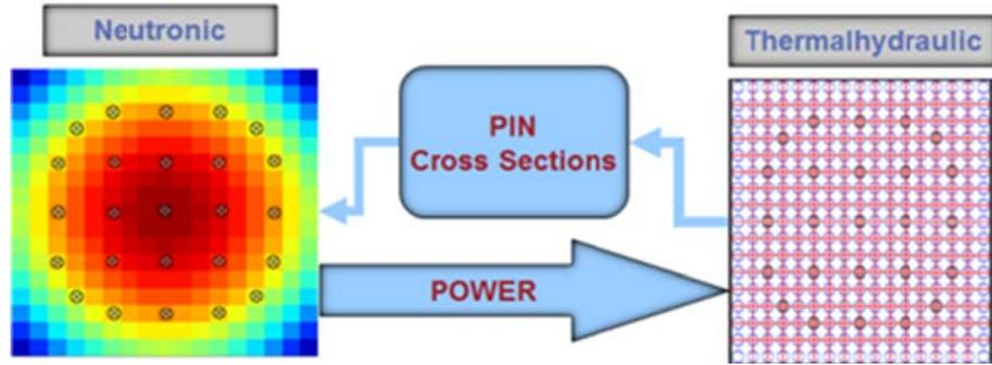
**Figure 6:** Interplay of neutronics (at core level, left) and thermalhydraulics (on fuel pin level in a fuel assembly-right) to be considered for pin-based multi-physics high fidelity computations.
