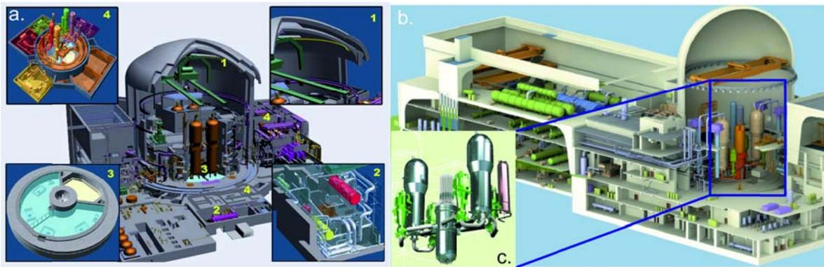
**Figure 13:** (a) Cut through the nuclear island of the EPR and safety systems installed. 1=double walled containment, 2= containment heat removal system, 3= corium spreading area and IRWST, 4=4 train safe guard system. b.) plant cut-away of the APR1400 by KEPCO and (c) primary circuit [21].
