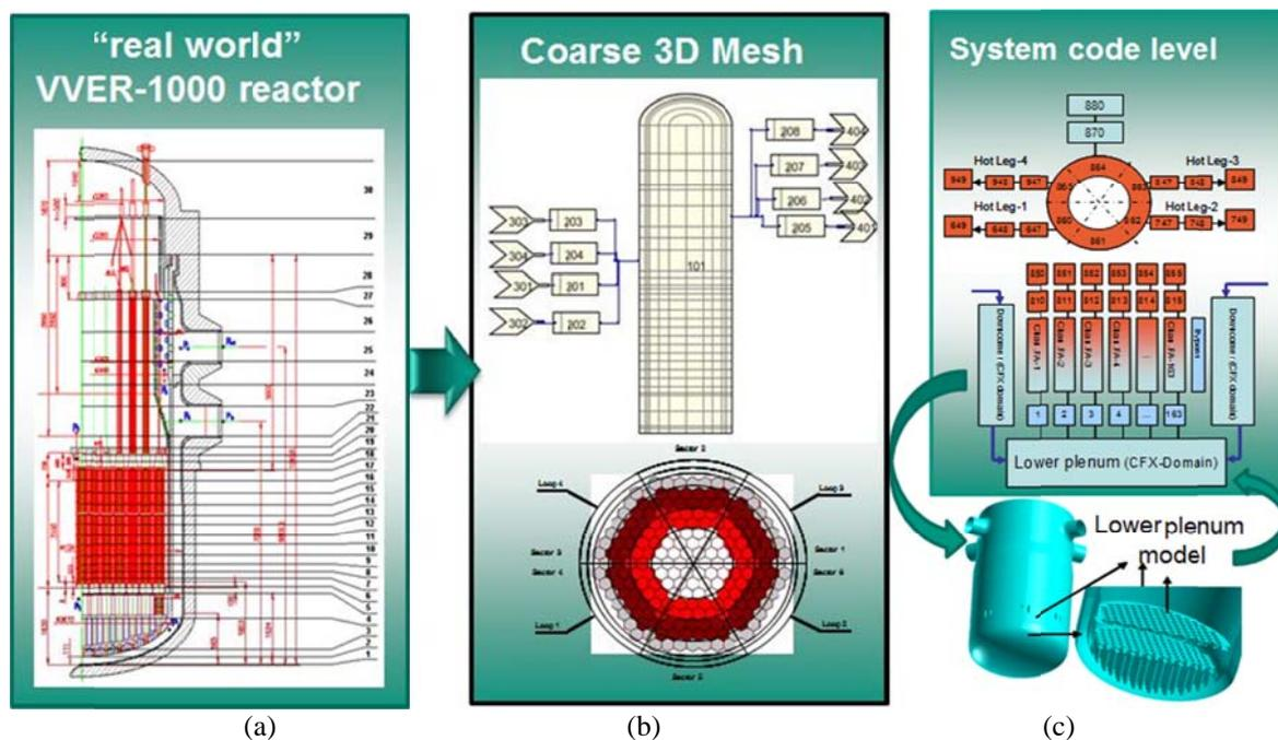
**Figure 2:** Transfer of reactor core (a) into nodal model (b) and then connection to thermal-hydraulic channels.
