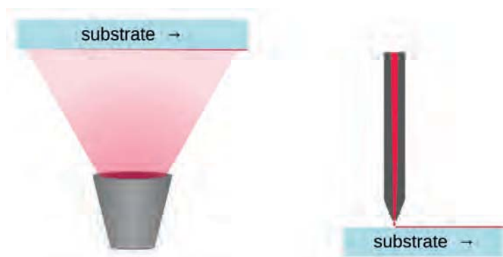
Fig. 2: Schematic illustration of the two dominant technologies for the deposition of organic semiconductors: thermal evaporation in vacuum (left) and solution processing by printing or similar techniques (right).
