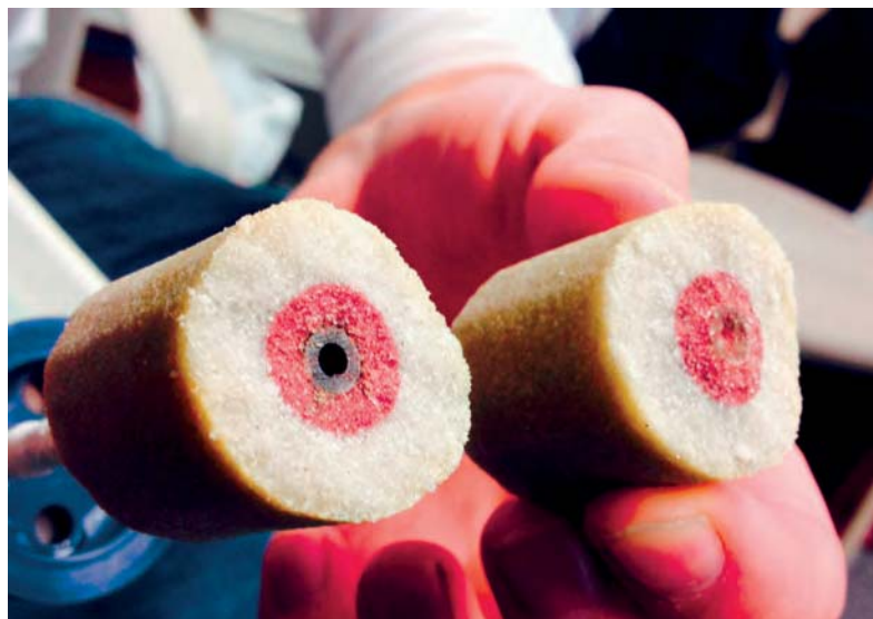
Fig. 11: Copper precipitation (orange rim) in an experimentally simulated rock-casing contact yielding clogging of pores and reservoir damage.
