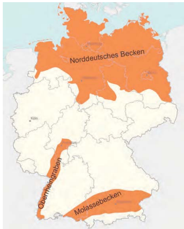
Fig. 2: German regions (orange) with the highest potential for geothermal energy supply.
