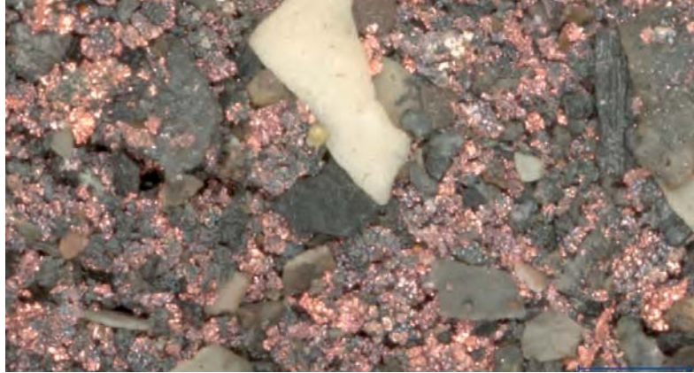
Fig. 10: Sediment recovered from the production well at the geothermal research platform Groß Schönebeck containing substantial amounts of native copper.
