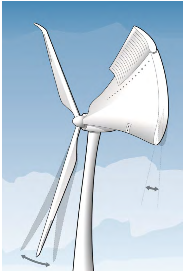
Figure 3: Scheme of a wind turbine with smart blades technologies [DLR]
