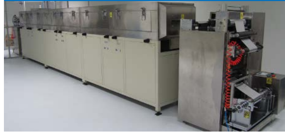
Coating and Drying
