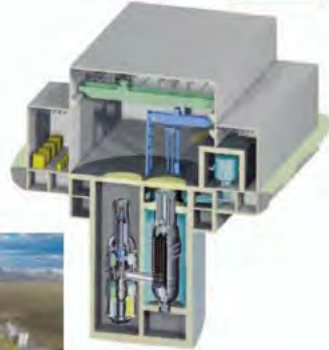
Figure 13: GENERAL ATOMICS – SMR: GT-MHR High Temperature Reactor (Source: GA, FRAMATOME)
