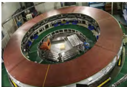
Fig. 11: The winding of 7 double pancakes for PF6 has been completed at ASIPP in Hefei. Nine double layers of conductor will be stacked to build the full coil, which is being built in China under contract with the EU-DA. (Source: F4E)
