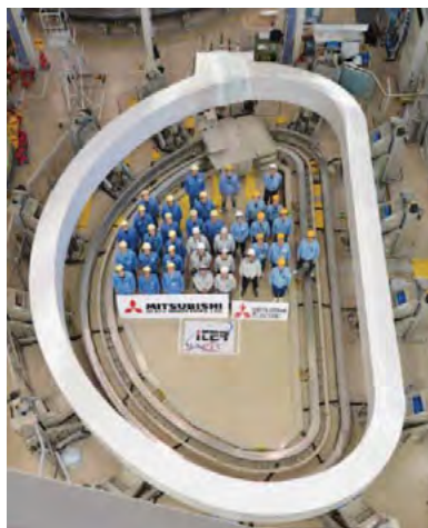
Fig. 10: The first complete toroidal field coil winding pack produced by Japanese industry (fabricated from Nb 3 Sn superconductor, with dimensions of 13.8 m x 8.7 m). (Source: Japanese DA)
