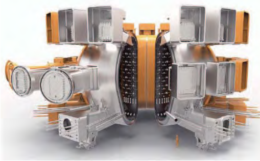
Fig. 4: Vacuum vessel (artist's view) The ITER vacuum vessel, a double walled, stainless steel structure with ~19.5 m outer diameter, ~11.5 m height and an overall weight of 5300 t. (Source: ITER)
