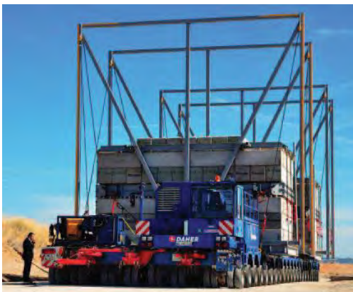
Fig. 9: Test transport for large components such as the toroidal field coils: a 352 wheel convoy carrying an 800 tonne dummy load, 33 m long, 9 m wide, 10 m high took 4 nights from Etang de Berre to the ITER site. (Source: ITER)
