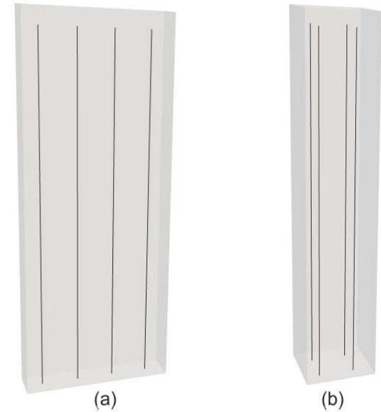
Figure 2: Multiple GSHP systems: a)  $1 \times 4$  arrangement, b)  $2 \times 2$  arrangement.
