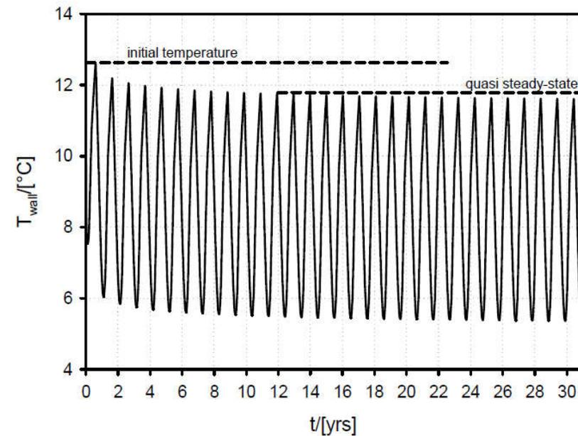
Figure 5: Temperature fluctuation at the BHE wall, measured at the top of the BHE. The initial and quasi steady-state temperatures are marked with dashed lines.
