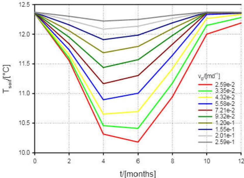
Groundwater flow - Subsurface temperature at a distance of 1 m beside the BHE
