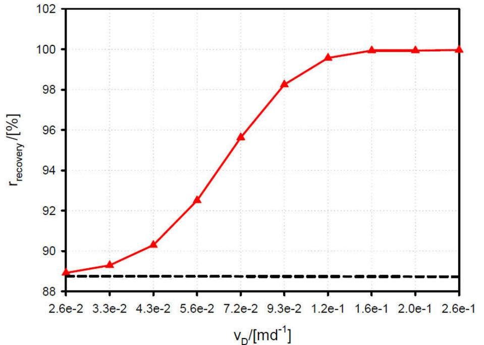
Groundwater flow - Recovery ratio as a function of Darcy velocity
