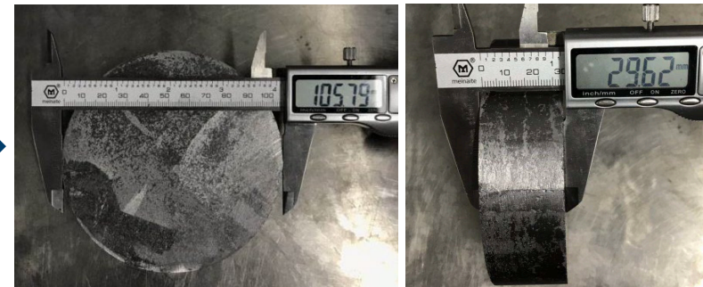
Porous W_f/W , 105 mm x 30mm, ~89% density, 40% fibers
