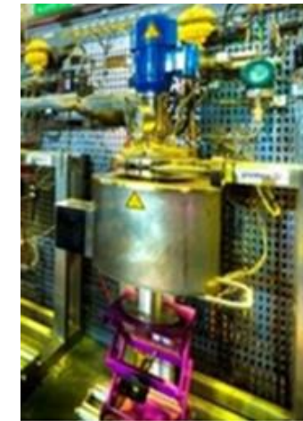
Micro-slurry reactor (10-20g catalyst) at industrially relevant conditions
